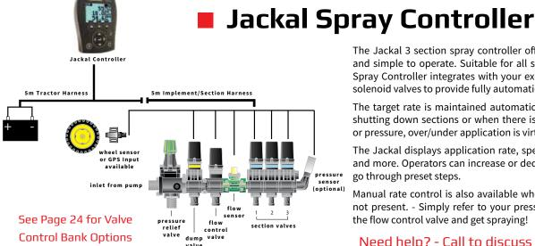
The Jackal 3 section spray controller offers great flexibility and simple to operate. Suitable for all sprayers, the Jackal Spray Controller integrates with your existing motorised or solenoid valves to provide fully automatic spray control.
